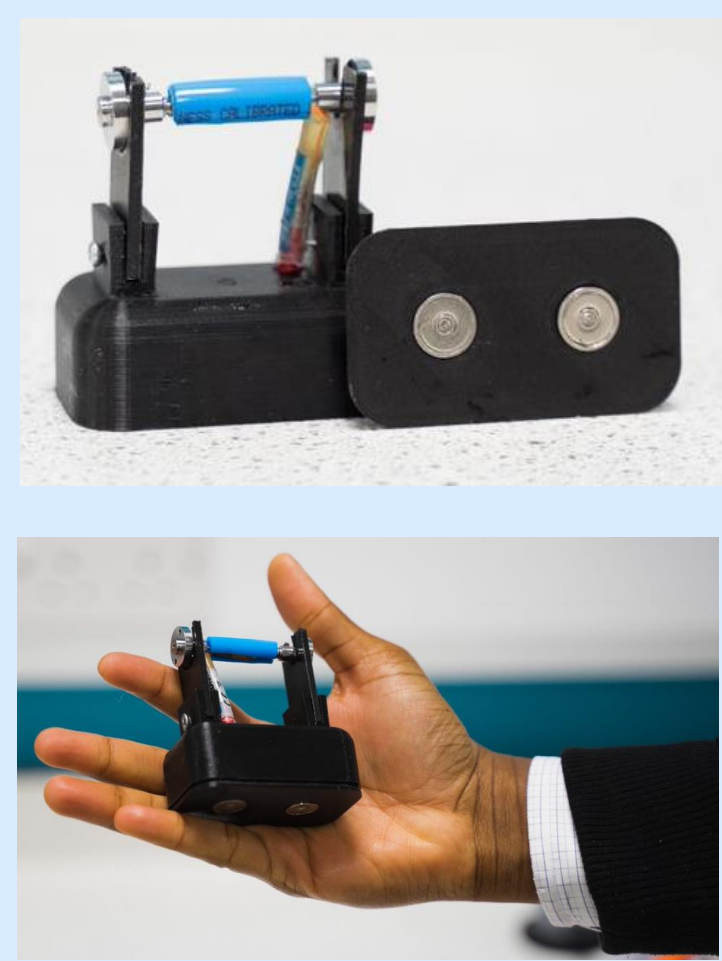
Magnetic box to host VWSG and wireless node
