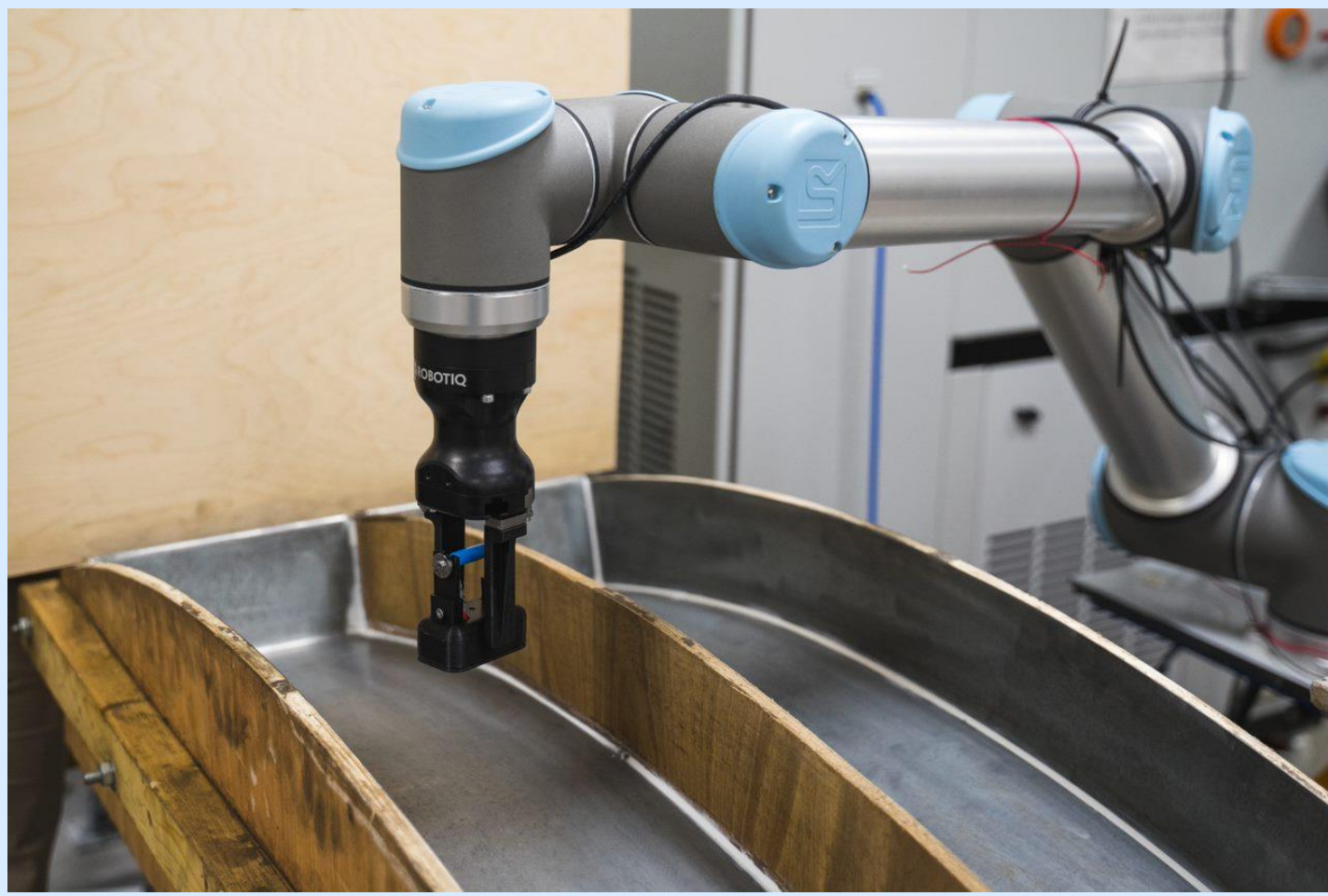
Pick-and-place of magnetic box using 6-axis collaborative robot before casting.
