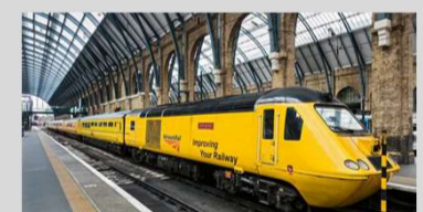
Network Rail's New Measurement Train for inspecting track quality with high precision.
