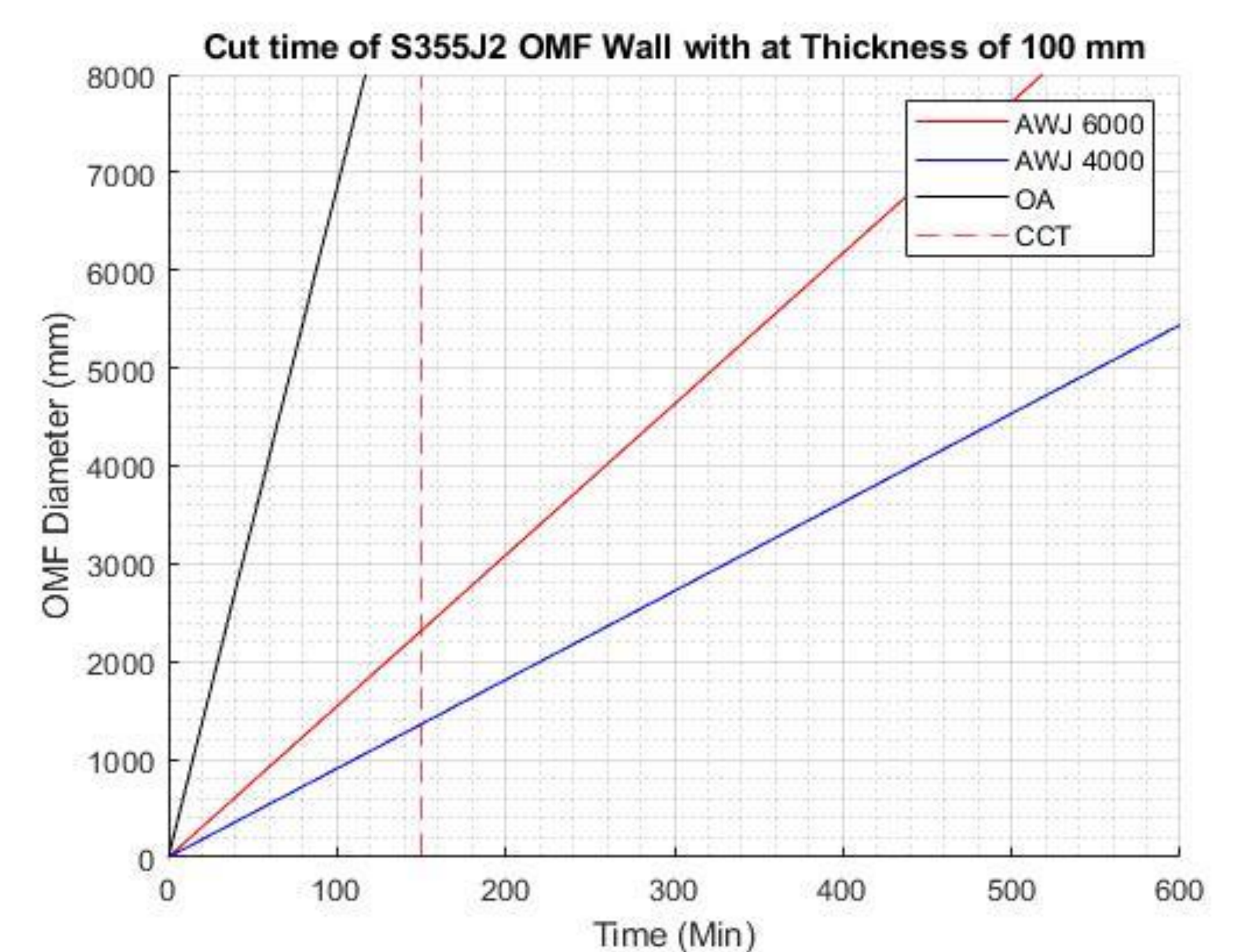
Figure 6 - Cutting time of EN 1.0577 (S355J2), applying Abrasive Water Jet (AWJ) 6000 bar, 4000 bar, Oxy Arc Torch (OA) and the Cooling Cutting Technique (CCT)
