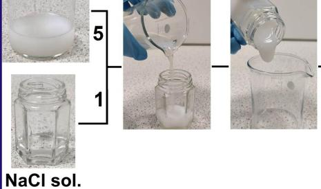
**2.** Colloidal Silica Grout
